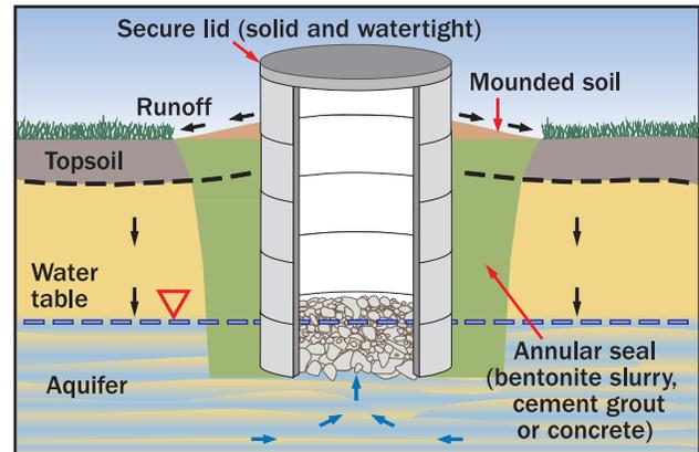
**Figure 1.** A properly constructed dug or bored well keeps surface water and contaminants from the well.
