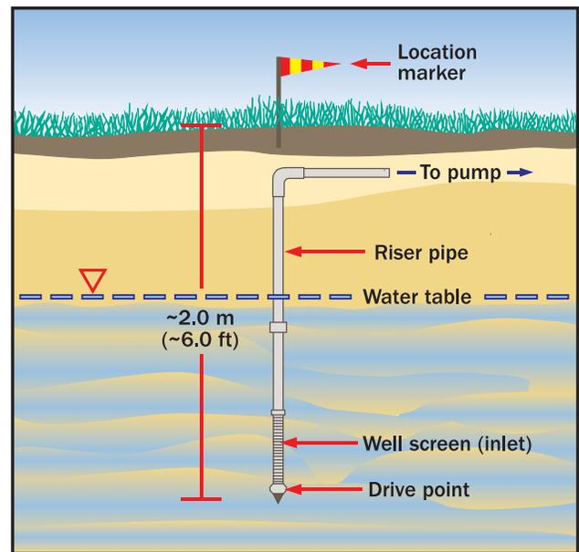
Figure 3. Example of a well point installation.
